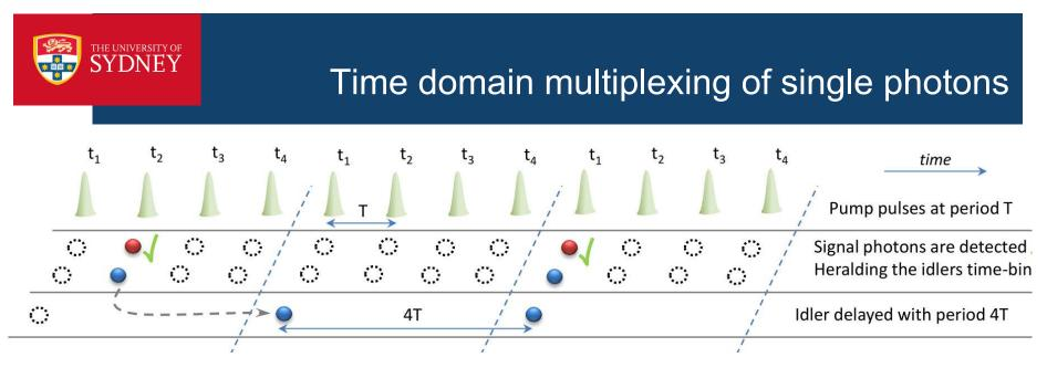
**Initially expectation** : Heralded single photon rate should enhance significantly without degrading coincidence to accidental ratio (CAR)
