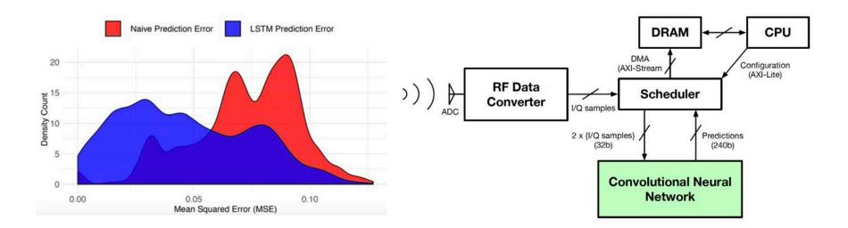
LSTM Spectral prediction: 4.3 µs latency on Ettus X310 XC7K410T (MILCOM'18) Ternary Modulation classifier: 488K class/s, 8us latency, Xilinx ZCU111 RFSoC (FPT'19)
