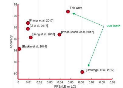
Ours is the most accurate and fastest reported FPGA-based CNN inference implementation CIFAR10: 90.9% acc, 122K fps (TRETS'19)
