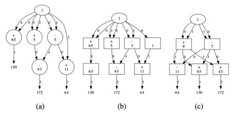
Fig. 1. Graph realizations of coefficient set  $\{44, 130, 172\}$ : (a) Adder graph obtained by  $H_{cub}$  AD min, (b) PAG using ASAP pipelining, (c) optimal PAG
