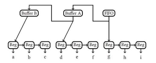
Input FIFO outputs the pixel each cycle to both Buffer A and the first stage of a shift register.
