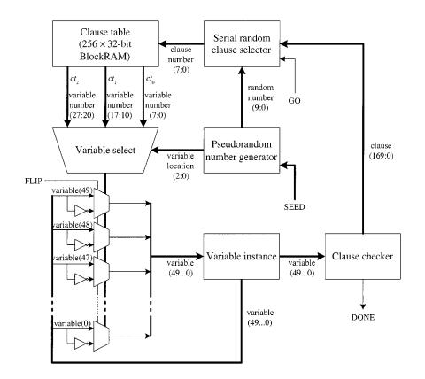
Fig. 1. Datapath of the WSAT core.
