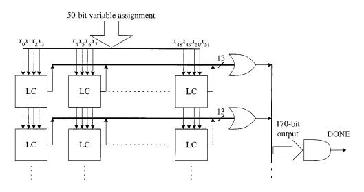
Fig. 2. Block diagram of the clause checker. Note that bits 50 and 51 are unused.
