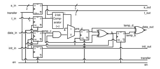
**Fig. 3.** The Smith-Waterman processing element (PE). Boxes represent D-type flip-flops.
