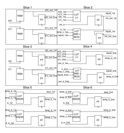
Fig. 4. Two processing elements mapped to 6 Virtex slices.
