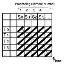
Fig. 2. Data dependencies in the alignment table. Thick lines show entries which can be computed in parallel and the time axis is arranged diagonally.
