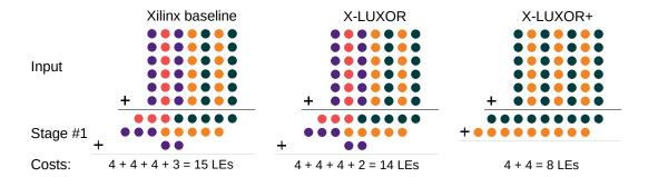
Figure 8: Example compressor tree for a 6-operand 7-bit addition using Xilinx baseline, X-LUXOR, and X-LUXOR+
