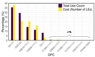
Figure 6: Total percentage count and cost of each GPC/compressor found in optimal solutions of compressor trees across 50+ Micro-Benchmarks from a variety of fields. The GPC/compressor list is according to [22]
