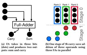
Figure 1: (3:2) parallel counter, also known as a full-adder.
