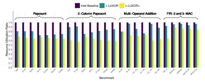
Figure 12: Resource reduction on Intel Stratix-10, I-LUXOR, and I-LUXOR+ architecture for our selected micro-benchmarks.
