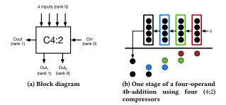
Figure 3: Simple (4:2) compressor example.
