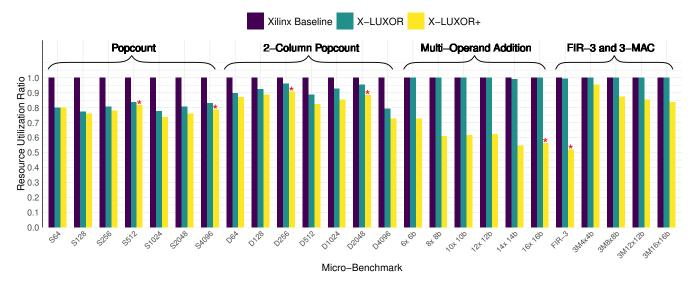
Figure 11: Resource reduction on Xilinx UltraScale+, X-LUXOR, and X-LUXOR+ architectures for various micro-benchmarks. The \* indicates that the proposed solution required one less logic stage in the compression tree.
