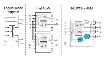
Figure 9: Efficient implementation of C25:121 GPC
