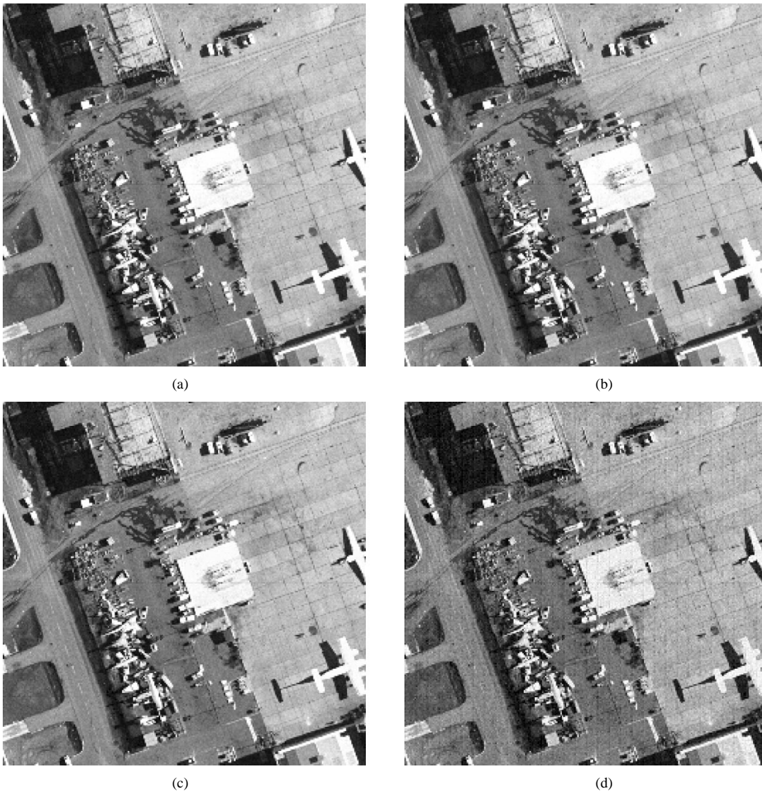
Fig. 8. Resultant images obtained from software fp and hardware fixed-point DCT image coding, followed by fp inverse DCT. Results from various algorithm performances are shown. The number of slices is measured in a bit-parallel implementation. (simulation SNR, actual SNR, slices). (a) Floating-point DCT. (b) Fixed-point DCT (251.811, 44.550 dB, 4013). (c) Fixed-point DCT (66.271, 32.520 dB, 751). (d) Fixed-point DCT (20.155, 19.664 dB, 651).
