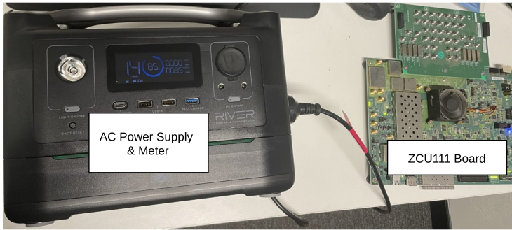
Fig. 18. Measuring the power consumption of the ZCU111 via AC power supply.
