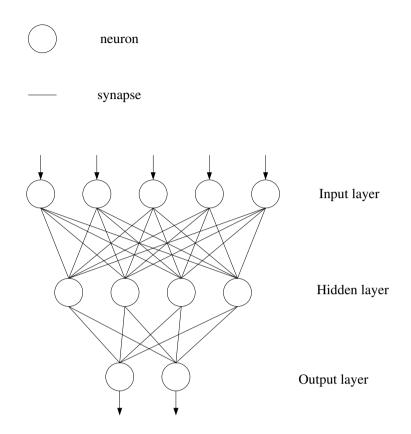
Figure 3.5: A three layer neural network architecture with five input nodes, four hidden nodes, and two output nodes.
