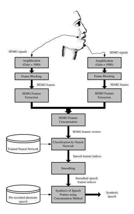
Figure 5.4: Speech synthesis from input SEMG signal.
