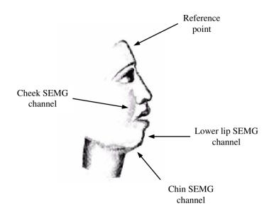
Figure 5.1: Electrode placement: SEMG signals were collected from the cheek, the chin, and lower lip, forehead was used as reference point.
