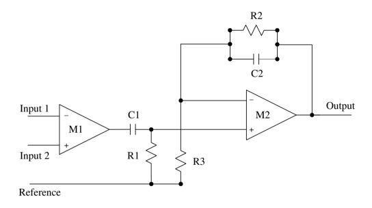
Figure A.1: Schematic circuit diagram of SEMG signal amplification. R1 =  $10k\Omega$ , R2 =  $100k\Omega$ , R3 =  $1k\Omega$ , C1 =  $1\mu$ F, C2 = 3.2nF, M1: Analog Devices AD625 amplifier, M2: Analog Devices AD210 amplifier.
