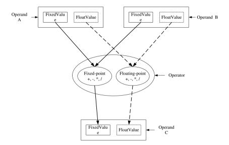
Figure 4.3: Arithmetic calculation using fixed-point object
