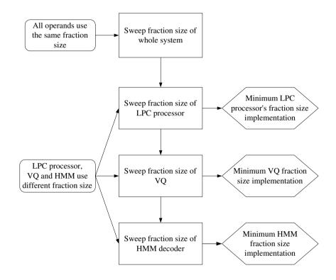
Figure 7.6: System level optimization using one-dimensional optimization
