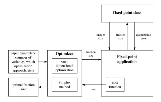
Figure 7.1: Block diagram of the framework
