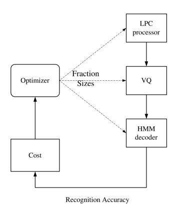
Figure 7.4: System level optimization using simplex method
