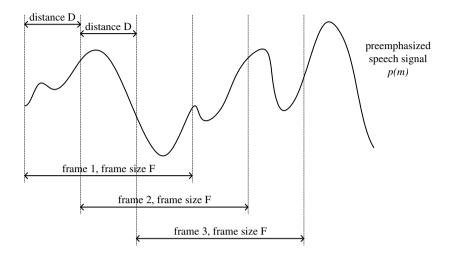
Figure 5.4: Frame blocking process
