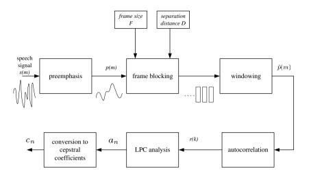
Figure 5.3: Block diagram of the LPC feature analysis
