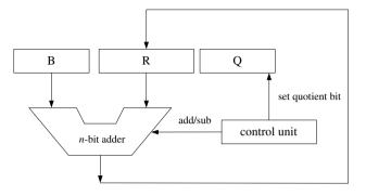
Figure 3.5: Block diagram of divider using restoring-division
