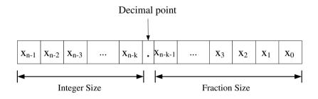
Figure 3.2: Fixed-point representation for fraction number
