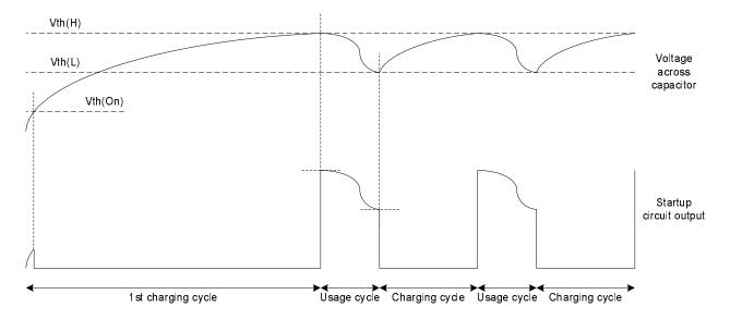
Figure 4.3: Output characteristics of startup module and system supply
