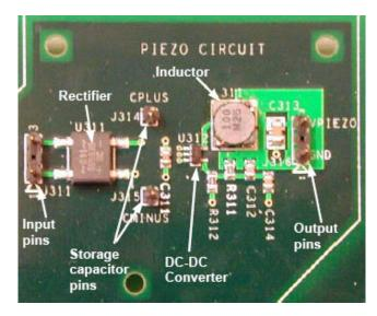
Figure 2.5: Photograph of power circuit of piezoelectric generator [40]. Photo courtesy of Shad Roundy
