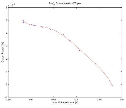
Figure 3.14: Output power versus input voltage of tripler
