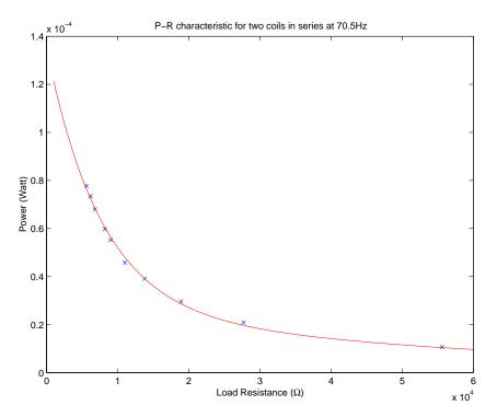
Figure 3.11: Output power versus load resistance for two MPG coils in series stimulated at 70.5Hz
