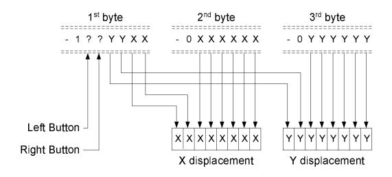
Figure 6.9: Data packet format for MS mouse protocol [10, 13]
