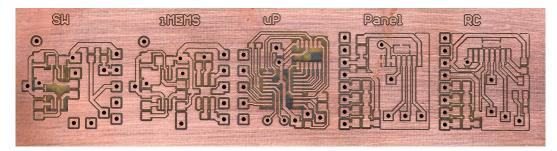
Figure 6.4: Rapid prototype of 2D Ring boards
