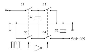
Figure 4.8: These essential components illustrate the mechanics of charge-pump operation. [34]
