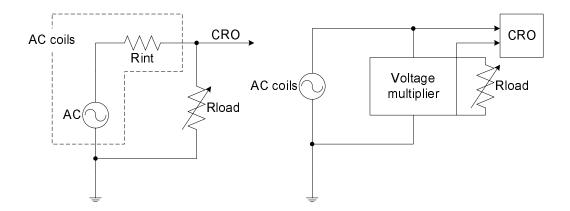
Figure 3.7: The experiment apparatus for measuring MPG coils characteristics.
