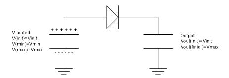
Figure 2.1: A simple circuit illustrates the idea of electrostatic power conversion [40].
