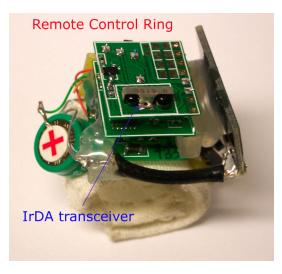
Figure 6.12: Photograph of 2D remote control ring
