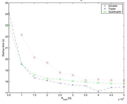
Figure 3.21: Startup time versus resistive load for  $V_{th}(H) = 1.4 V$  (simulated by PSpice)
