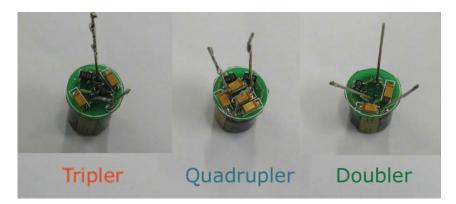
Figure 4.5: Voltage multipliers: tripler, quadrupler and doubler
