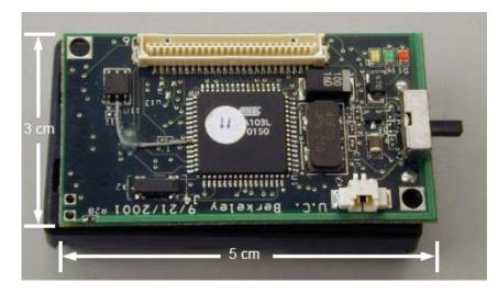
Figure 2.7: Photograph of MICA node [40]
