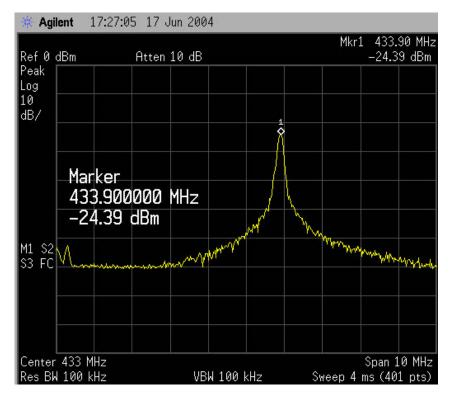
Figure 6.13: Transmission power of the 2D ring at 1 cm
