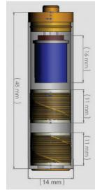
Figure 3.9: Illustrative drawing for micro power generator. Photo courtesy of Johnny M. H. Lee
