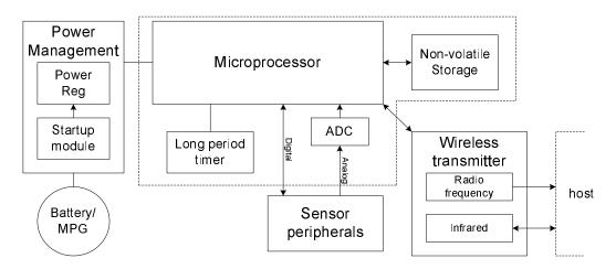
Figure 4.1: Generic platform block diagram
