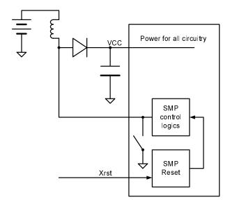
Figure 4.7: Programmable System on Chip has built-in switching regulator [26]
