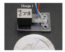
Figure 2.3: Photograph of Roundy's piezoelectric generator (Design 1) [40]. Photo courtesy of Shad Roundy
