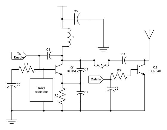
Figure 4.11: Schematic of SAW-based On-Off Keying RF transmitter [36]
