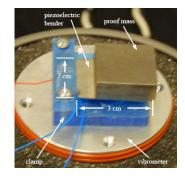
Figure 2.4: Photograph of Roundy's piezoelectric generator (Design 3) [40]. Photo courtesy of Shad Roundy
