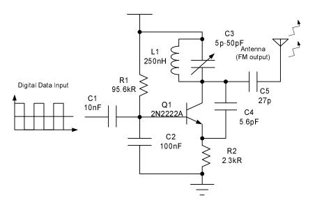
Figure 4.9: Schematic of LC-based radio frequency transmitter
