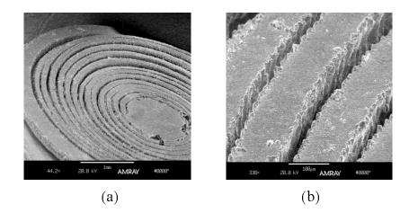
Figure 3.2: SEM pictures of: (a) a laser-micromachined copper spring with diameter of 5 mm, (b)close-up of the copper spring; width of spring is ~ 100  $\mu$ m. Photo courtesy of Johnny M. H. Lee.
