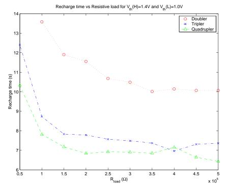
Figure 3.24: Recharge time versus resistive load for  $V_{th}(H) = 1.4 V$  and  $V_{th}(L) = 1.0 V$  (simulated by PSpice)
