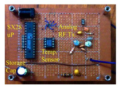
Figure 5.2: Photograph of prototype 1
