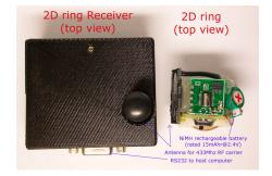
Figure 6.17: Photograph of 2D ring demo kit (top view)
