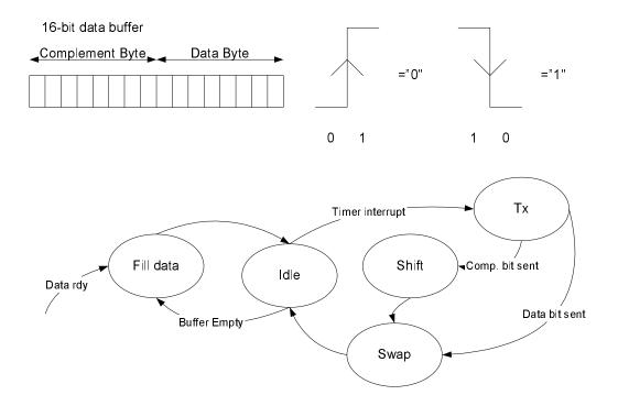
Figure 6.6: State diagram explains Manchester encoding
