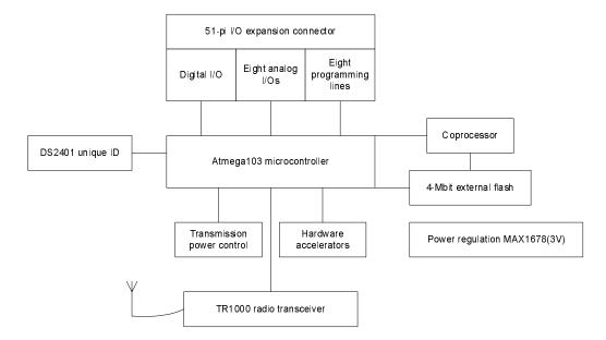
Figure 2.6: Block diagram of MICA node [14]
