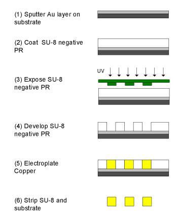
Figure 3.3: Copper spring fabrication process. Photo courtesy of Johnny M. H. Lee
