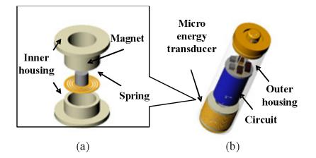
Figure 3.1: Illustrations of: (a) Inner structure of the micro power generator; (b) the AA-size micro power generator which is integrated with a power-management circuit. Photo courtesy of Johnny M. H. Lee
