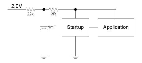
Figure 5.8: Setup for measuring power consumption of the startup and application circuit
