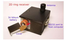
Figure 6.16: Photograph of 2D ring receiver
