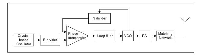
Figure 4.10: System block diagram of PLL with crystal
