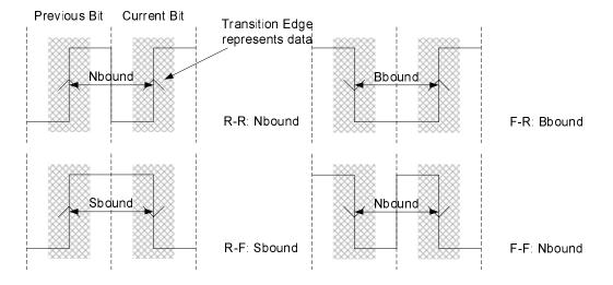
Figure 6.7: Timing diagram 1 explains Manchester decoding
