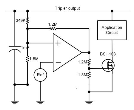
Figure 4.4: Schematic of startup module
