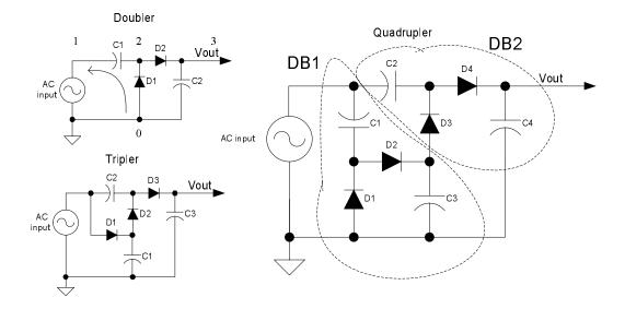
Figure 3.4: The schematics of voltage doubler, tripler and quadrupler [15]
