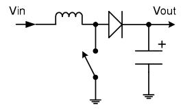
Figure 4.6: Simple boost converter [33]
