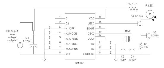
Figure 2.9: Wong's Infrared system block diagram [5]
