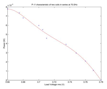
Figure 3.13: Output power versus load voltage of two MPG coils in series stimulated at 70.5Hz
