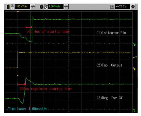
Figure 5.7: CRO screen capture for system startup
