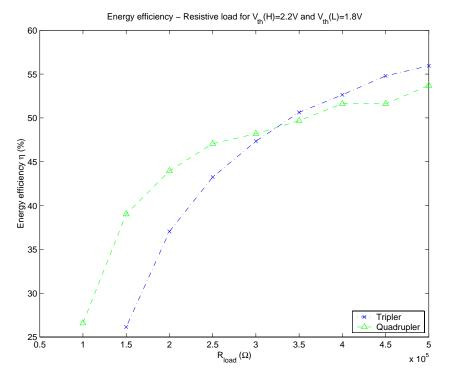
Figure 3.20: Energy efficiency versus resistive load for  $V_{th}(H) = 2.2 V$  and  $V_{th}(L) = 1.8 V$  (simulated by PSpice)
