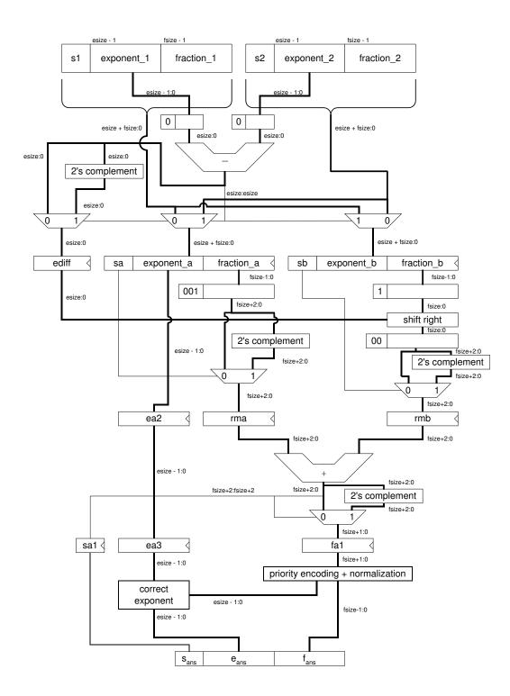
Figure 5.3: Parameterized Floating Point adder datapath
