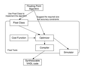
Figure 5.1: Floating point algorithm design flow.
