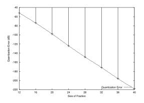
Figure 7.3: Quantization error for different fraction sizes.
