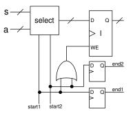
Figure 4.1: Circuitry used to handle multiple assignments to the same variable. This is the circuit which results from a program with two assignments  $l=\a$  and  $l=\s$ .
