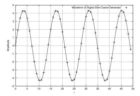
Figure 7.1: Digital sine-cosine generator reference output.
