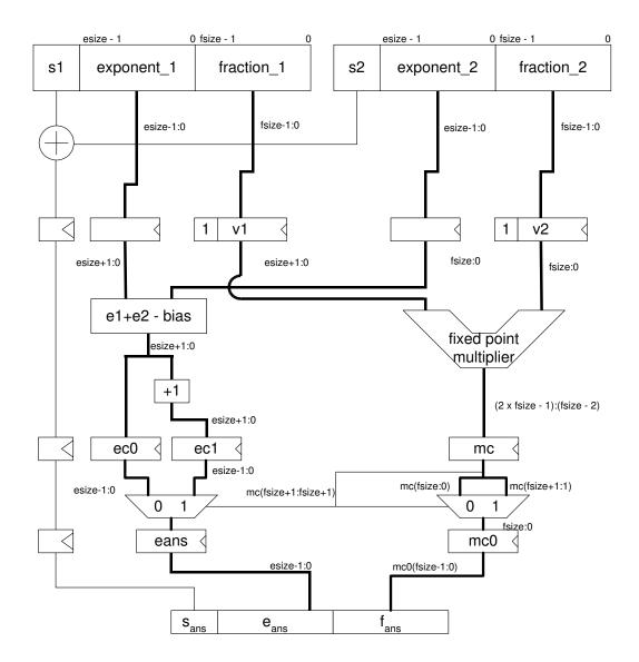
Figure 5.2: Parameterized Floating Point multiplier datapath
