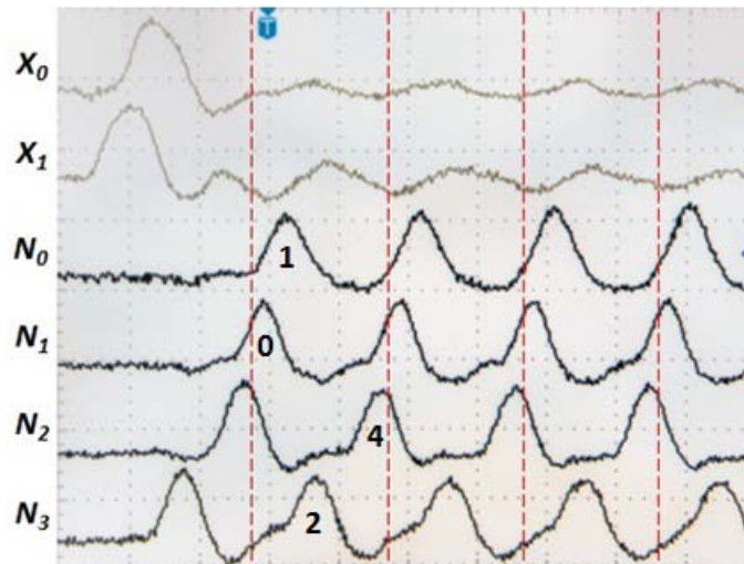
Figure 4.13: Recall of pattern \{1, 0, 4, 2\} captured on oscilloscope; voltage 5V/div, time 10ns/div
